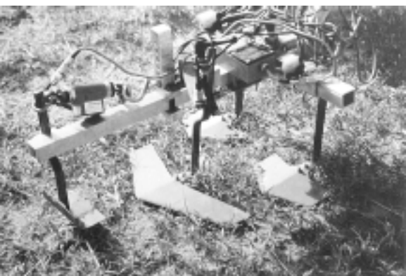
Figure 2c: Experimental weeder with 120° blades
